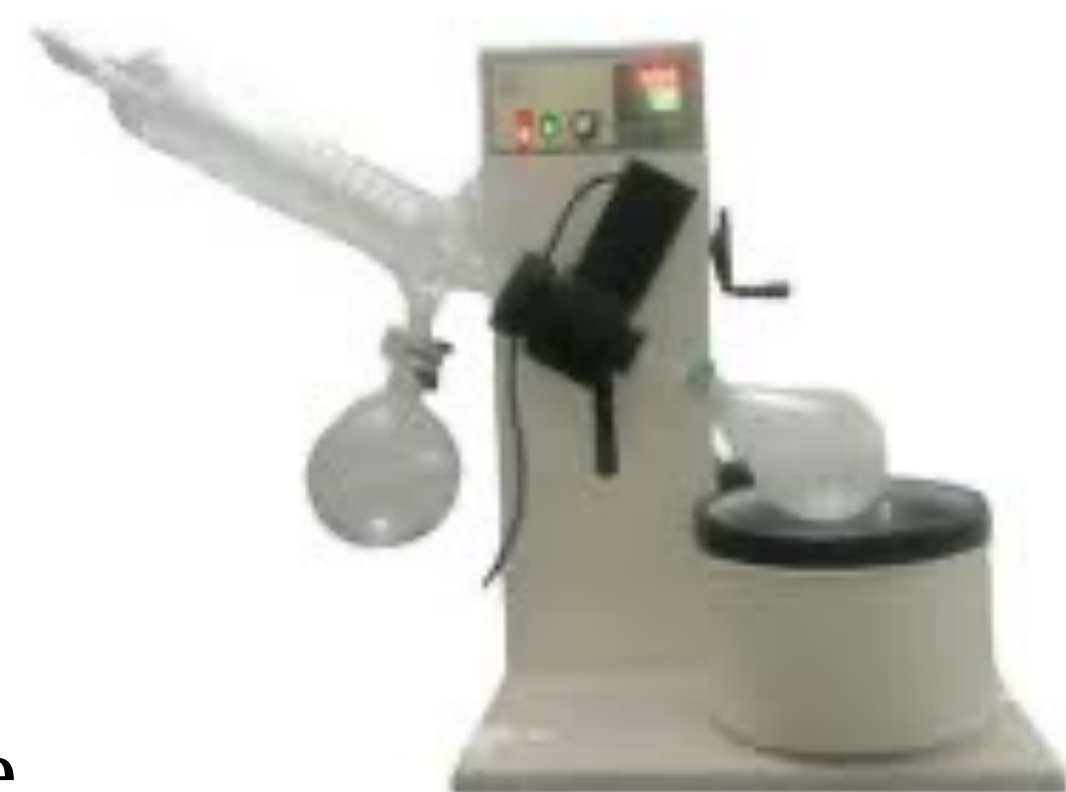
Figure 2. Model of a Rotary Evaporator.
